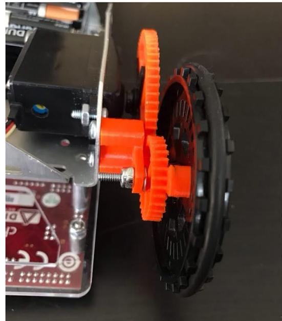
The pictures above show the assembled gear system (shown with medium gear attached).
