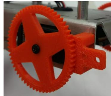
The next step in the assembly process is to attach the gears (either medium OR small) to the wheels and then to the slot on the mounting plate. The small and medium gears are designed with arms that fit into slots in the wheel providing additional points of attachment. This part of the assembly process will assume we chose to use the small gear.
