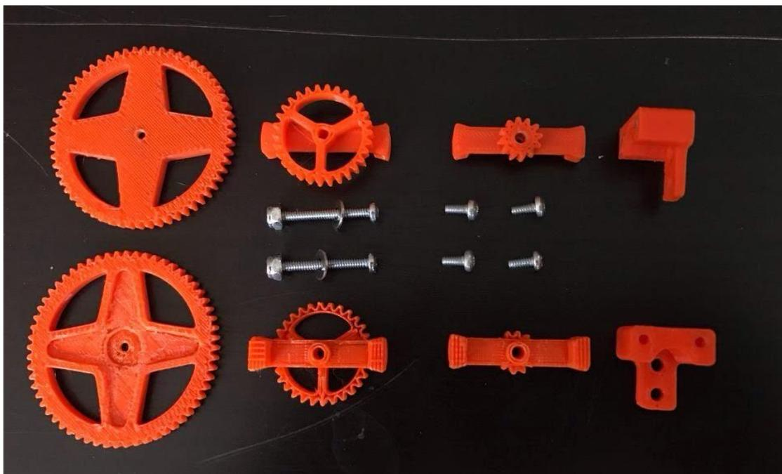
None of the additional parts were created with threading, all of them will need to be threaded using the screws provided. There are a total of 2 mounting plates, each with 2 holes for mounting onto the robot and 2 holes used for mounting the small or medium gears.
