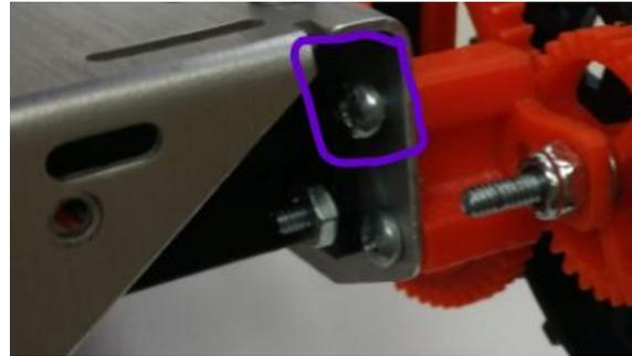
The wheel mounting slots of the mounting plates should be pointed away from the robot frame.
