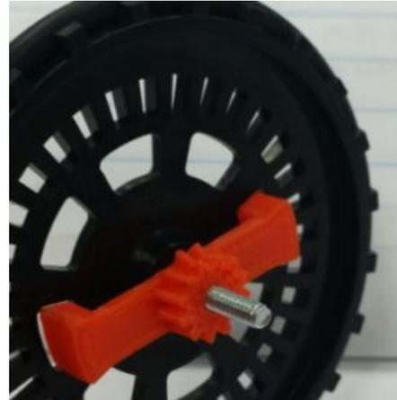
Once the gear system is assembled and the robot is ready to run, the code for the servo speeds must be made negative so that the wheels will run in the forward direction. If not, the robot will run in reverse. Alternatively, the servo motors could be swapped, left to right. In this case the plug-ins for the servos would also need to swap positions on the plug-in board.
