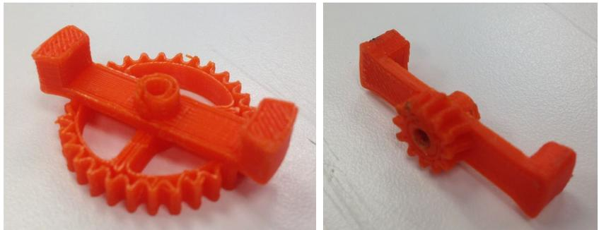
Finally, to minimize the amount of material needed to print the gear assembly, we cut out sections of material from the body of our gears, switching from a solid design to a spoked design. This modification did not alter the performance of our gears, but simply eliminated material, thus reducing the overall cost of the assembly.
