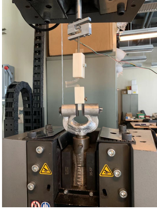
Figure 2.18: Schematic of the experimental setup to measure the fracture toughness of the SEBS soft tissue simulants. Trouser tear test is used to measure the fracture toughness of the SEBS soft tissue simulants to mode I crack propagation.
