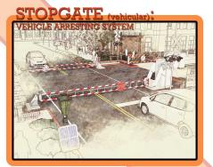
The StopGate is an advanced alternative to the conventional automated gates, designed to block out-of-control vehicles from entering the right-of-way. The StopGate's energy absorbing steel cables absorb the force of a runaway vehicle, compelling even a three-ton truck traveling 45mph to come to an immediate halt. Prior to the StopGate system, there was no remedy to immobilize runaway vehicles, except with tunnels and bridges, which cost millions of dollars. millions of dollars.
