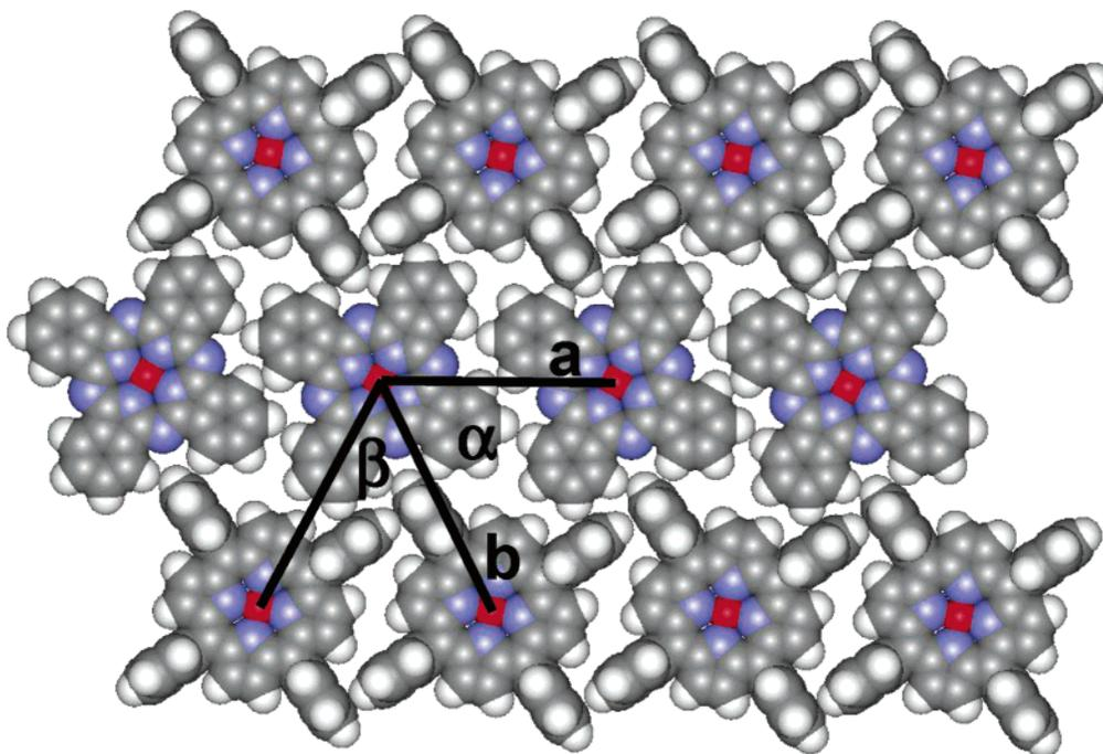
**Figure 8.** Model of the preferred surface structure of the mixed regions. Lattice spacings are  $a = 1.35 \pm 0.15$  nm along rows with nonalternating molecules and  $b = 1.50 \pm 0.15$  nm along rows with alternating molecules. Two different angles are possible between adjacent rows. The angle  $\alpha$ , between rows with alternating and nonalternating molecules, is  $63 \pm 5^\circ$ . The angle  $\beta$ , between two rows with molecules that alternate, is  $54 \pm 5^\circ$ .
