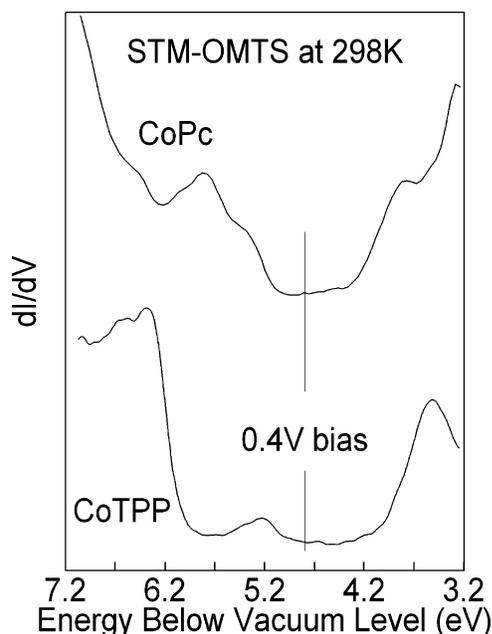
**Figure 9.** STM-OMTS of CoPc and CoTPP at 298 K. Zero bias is taken as 5.2 eV relative to the vacuum level. The bias at which Figure 6 was acquired (+0.4 V) is indicated on the graph.
