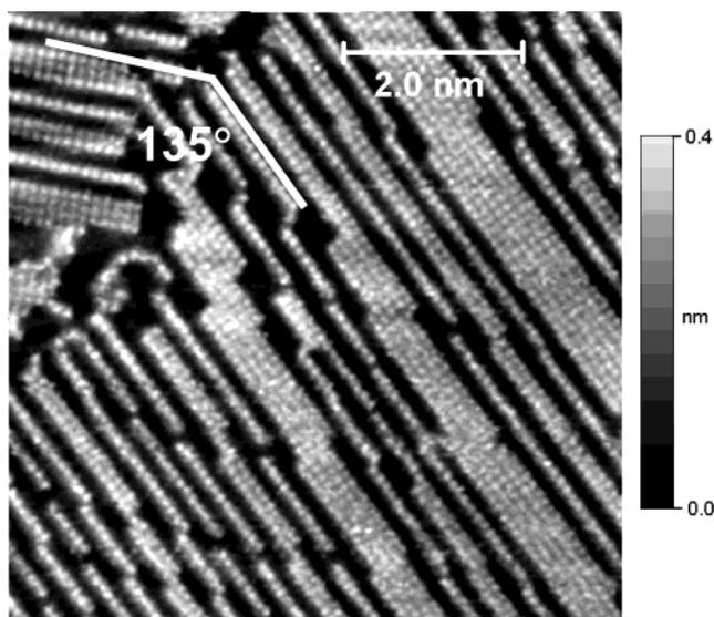
**Figure 6.** Approximately 0.7 ML of the pure CoPc/Au(111) sample in a region with the one-dimensional rows. Acquired at 295 K with a W tip,  $+0.8$ -V sample bias, and 0.1 nA setpoint. The image was flattened.
