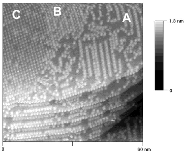
**Figure 5.** STM constant-current image of a CoPc/CoTPP mixture at  $T = 176$  K. A total of 0.3 ML of CoPc was first deposited on Au(111) followed by 0.5 ML of CoTPP. The image was acquired using a W tip at setpoint with a  $-0.8$ -V sample bias and 0.1 nA and was flattened. The top portion of the image shows distortion due to piezo creep.
