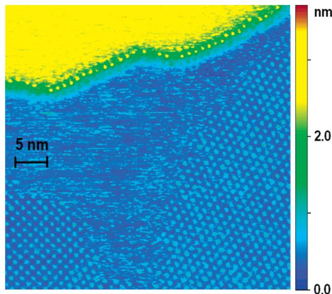
**Figure 4.** STM constant-current image of a CoTPP/CoPc mixture,  $T = 295$  K. A total of 0.25 ML of CoTPP was first deposited on Au(111) followed by 0.3 ML of CoPc. Acquired with a W tip at a setpoint with a  $-0.4$ -V sample bias and 0.10 nA.
