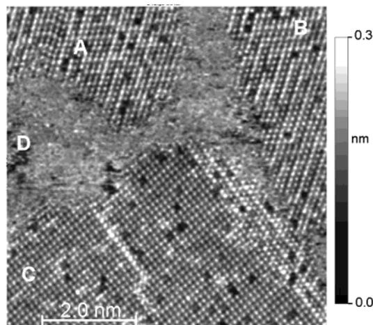
**Figure 3.** STM constant-current image of a CoPc/CoTPP mixture,  $T = 295$  K. A total of 0.3 ML of CoPc was first deposited on Au(111) followed by 0.5 ML of CoTPP. Acquired with a Pt/Ir tip at a setpoint with a  $-0.8$ -V sample bias and 0.05 nA. The image was flattened.
