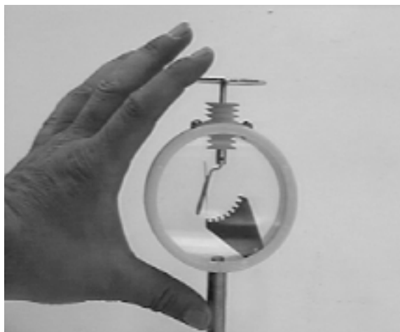
Figure 1.1. “Grounding” the electroscope.
