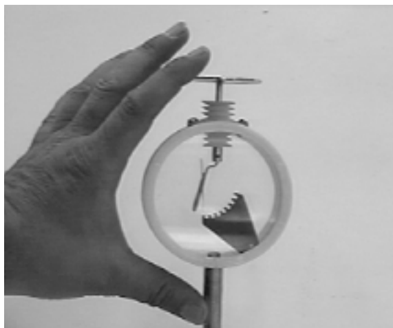
Figure 2.1. “Grounding” the electroscope.
