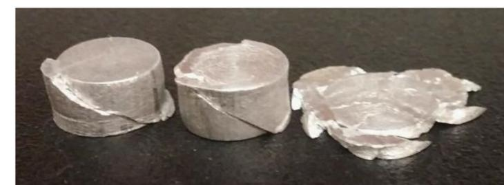
.001 strain rate, 600 strain rate, 2000 strain rate from left to right
