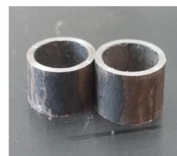
10% strain stopper and 3% strain stopper from left to right
