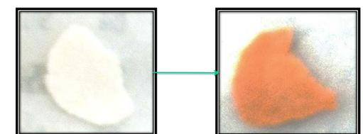
Fig. 6. Selenium dioxide pellets. Left image shows sample before being placed in FTIR vacuum chamber. Right image is of sample after 2 days in FTIR vacuum chamber.
