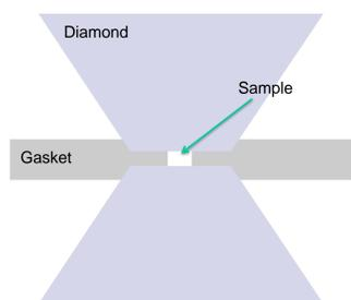
Fig. 1. Diagram of diamond anvil cell (DAC)
