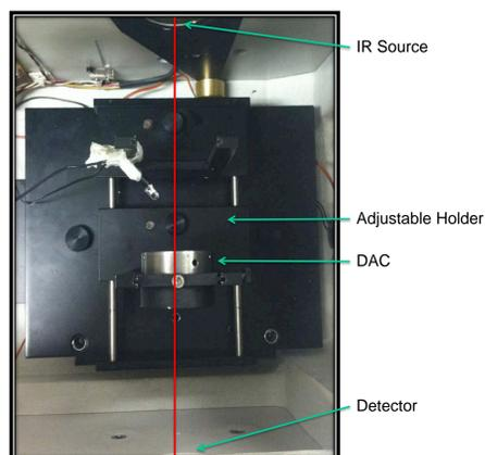
Fig. 3. Setup in FTIR vacuum chamber
