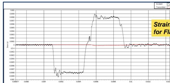
Strain Gauge Data for Flat Plate HDPE
