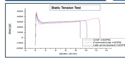
The top left plot shows the commercial HDPE flat plate sample tested at different strain rates. The top right plot shows two different materials (CNF-HDPE and commercial HDPE) tested at the same strain rate of 2000/s. The bottom plot shows the three materials (CNF-HDPE, commercial HDPE, and lab-processed HDPE) tested with the static tension test.
