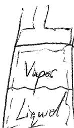
system  $\Rightarrow$  If system is in equilibrium with 2 phases it is in a saturated state.  $T \& P$  are not independent in 2-phase region, therefore we need another type of property.
