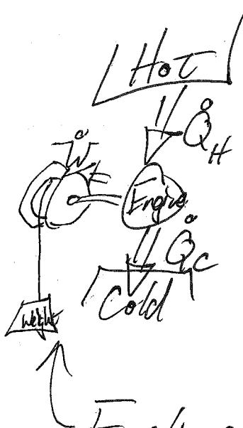
Thermal reservoir: infinite temperature source, provides thermal energy  $Q$  @ a constant temperature during the process under consideration: Lakes, rivers, atmosphere, buildings etc.
