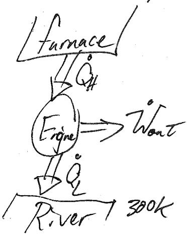
$$\eta_{\text{Thermal}} = \frac{W_{\text{out}}}{Q_H} = \frac{Q_H - Q_L}{Q_H} = \frac{80 \text{ MW}}{80 \text{ MW}} = 0.375 \text{ or } 37.5\%$$
