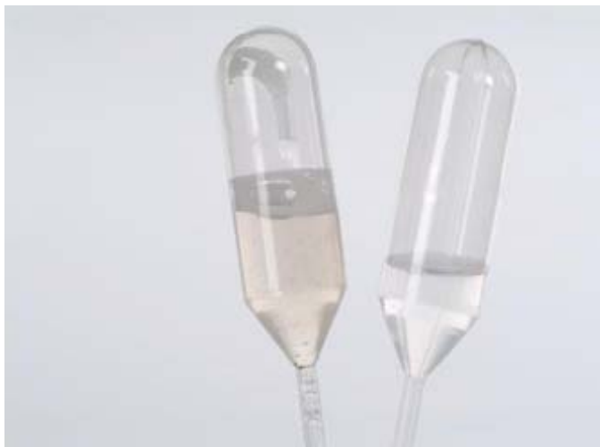
4 a) Check to see if the extraction liquid is discoloured
