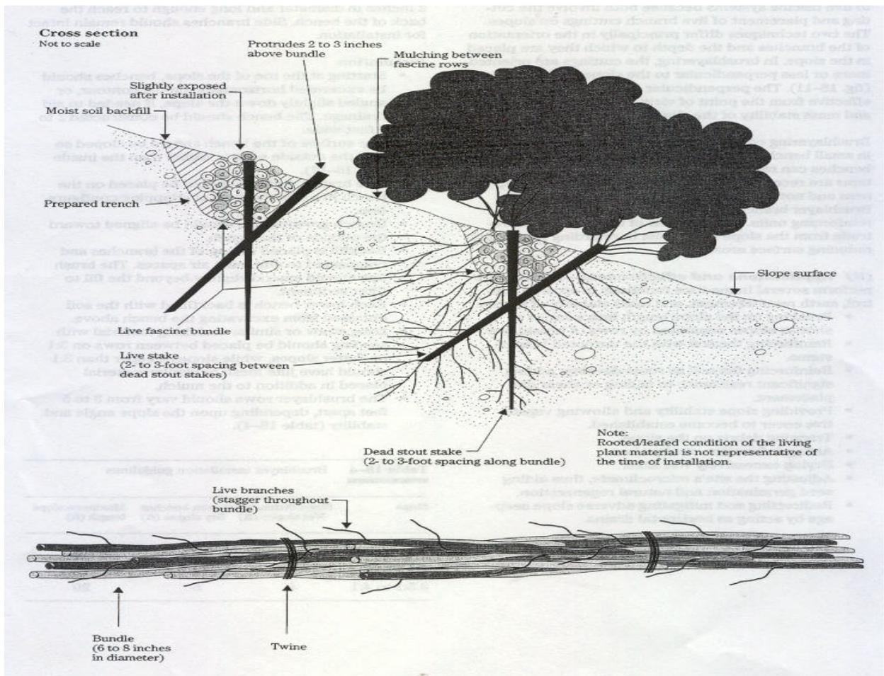
**Figure 1: Installation of Fascines**
