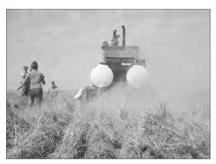
Fig. 1. WSU Lind drill with shovel-type openers on two ranks. This prototype has a 17-inch row spacing, solid packer wheels, and the frame is located high off the ground to allow clearance of high quantities of residue. We have had no plugging problems with this prototype in two years of testing.
