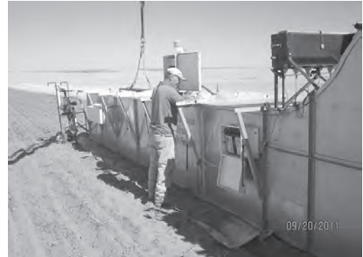
Fig. 1. A portable wind tunnel was used to measure soil sediment flux and PM 10 emissions, shown here at the Ron Jirava farm near Ritzville.
