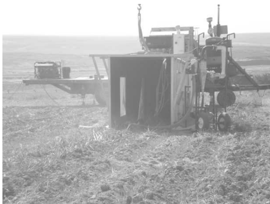
Fig. 1. Wind erosion assessed using a wind tunnel after sowing winter wheat at Lind, WA in August 2011.
