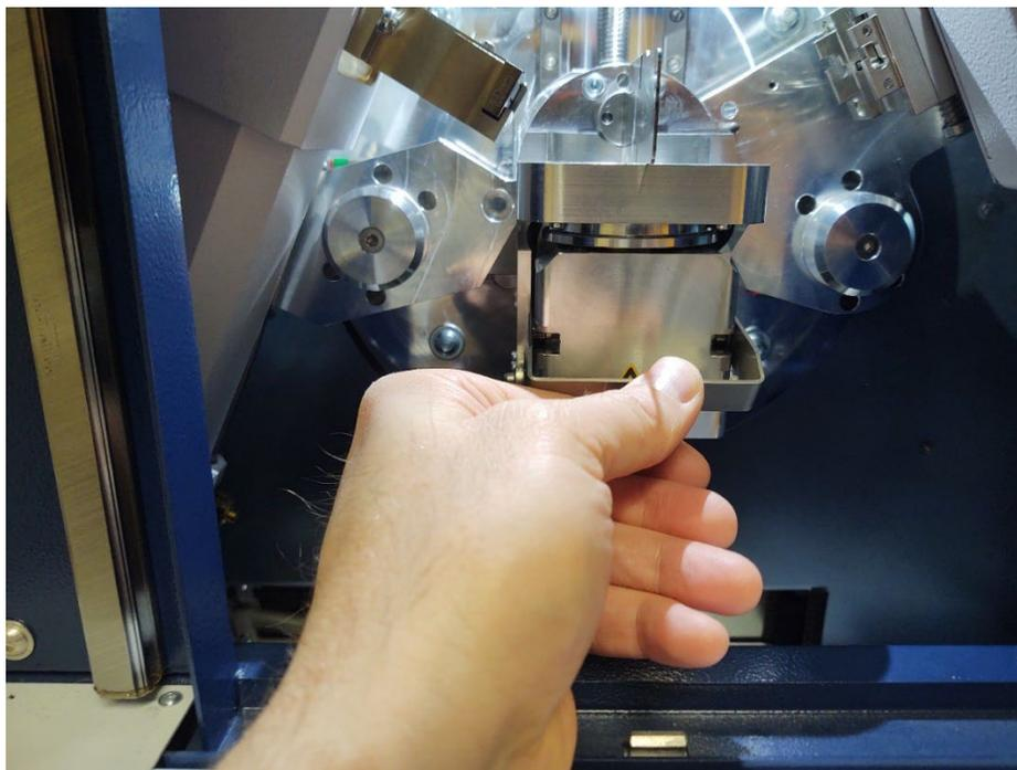
4.34 After the sample has been removed, clean up any mess left over from the sample and close the door, leaving the sample holder in the down position.
