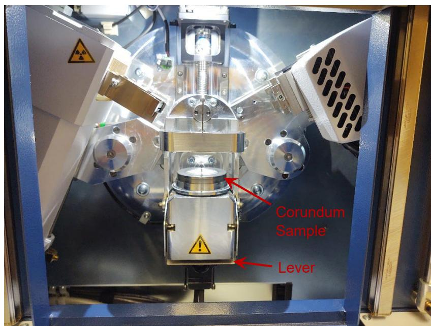
6.14 The sample is then moved into place by lifting the lever underneath the sample holder.
