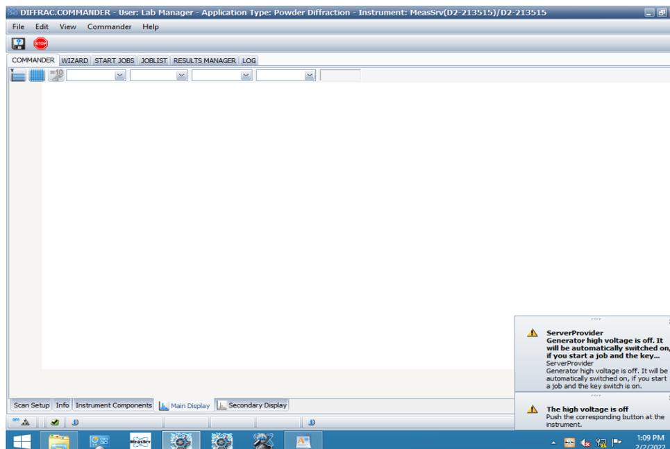
6.21 To set up a scan, click on the Scan Setup tab on the bottom of the Commander window to see the data collection parameters.
