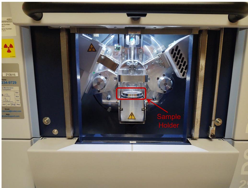
6.13 The picture shown below demonstrates the instrument with the corundum standard sitting on top of the sample holder, prior to moving the sample up into the measure position.
