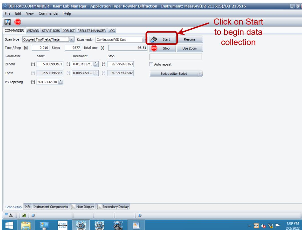
6.31 Upon clicking on start, you will hear a click and the yellow lights on top of the instrument will illuminate. A red light on the left side of the instrument will also illuminate, indicating that the X-rays are on.
