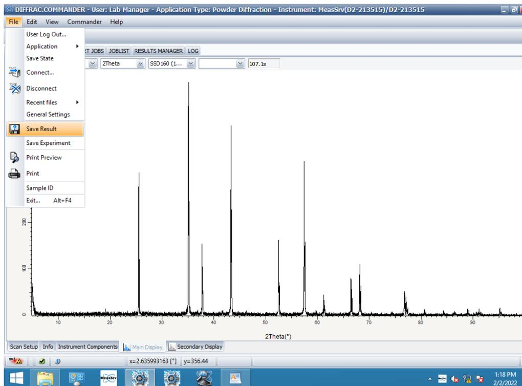
6.35 The save options are .brml file which is a Bruker diffraction data file that is only readable by the PXR software. The .raw file can be used with other X-ray diffraction programs. The data can also be saved as a .txt file for analysis in Origin or Excel.
