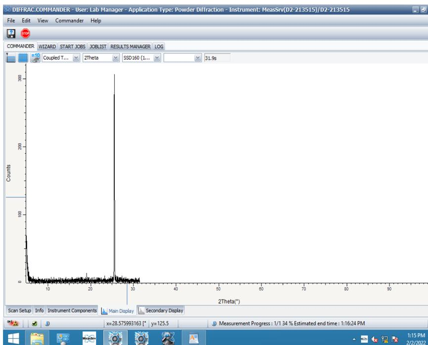
6.33 When the scan has completed, you will see a note on the bottom right of the window saying: Job finished” You will also see that the Busy light on the left side of the instrument is no longer illuminated.
