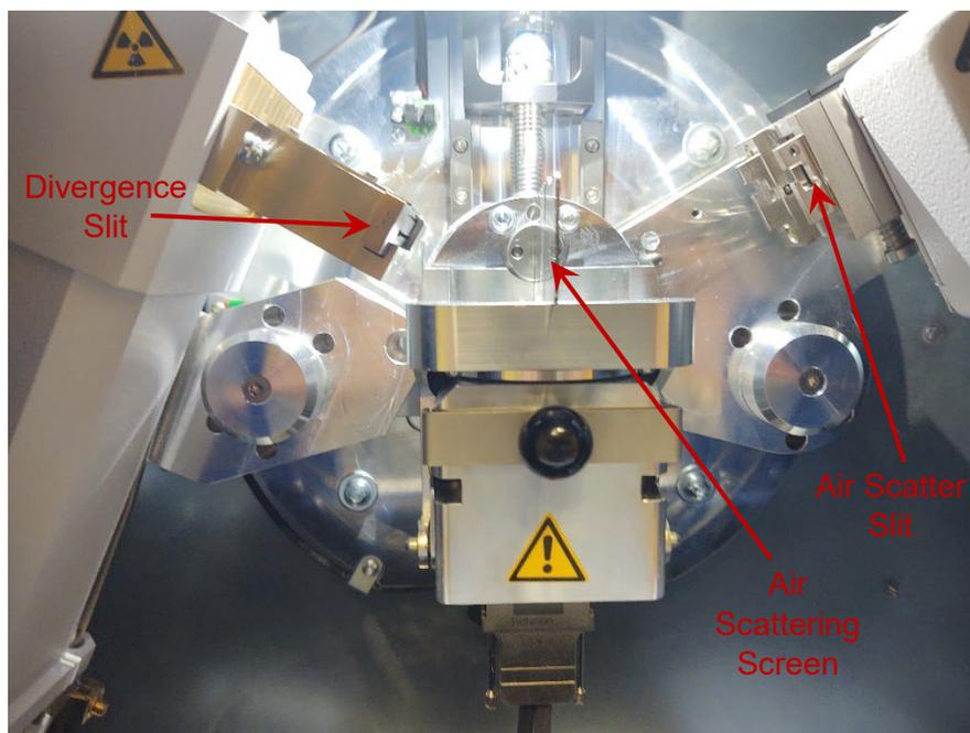
6.15 Before closing the instrument, the divergence slit, the air scattering screen, the Soller slit, kβ filter, and the air scatter slits need to be adjusted, if needed. Usually just the Divergence Slit and Air Scattering Screen need to be adjusted.
