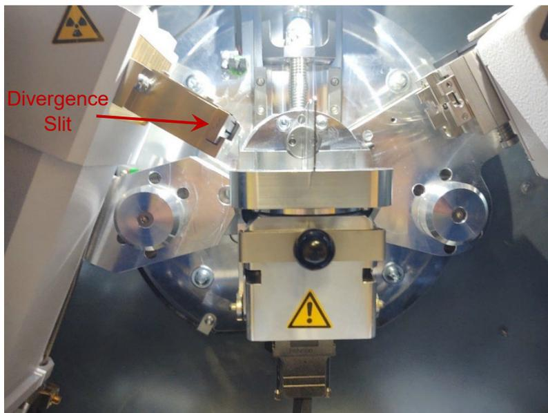
6.18 The air scatter screen can either be set to 1 mm or 3 mm. It is changed by pulling it off and having the desired screen facing down. The air scatter screen in the picture is set to 3 mm. The air scatter screen connects to the instrument with magnets and should click into place.
