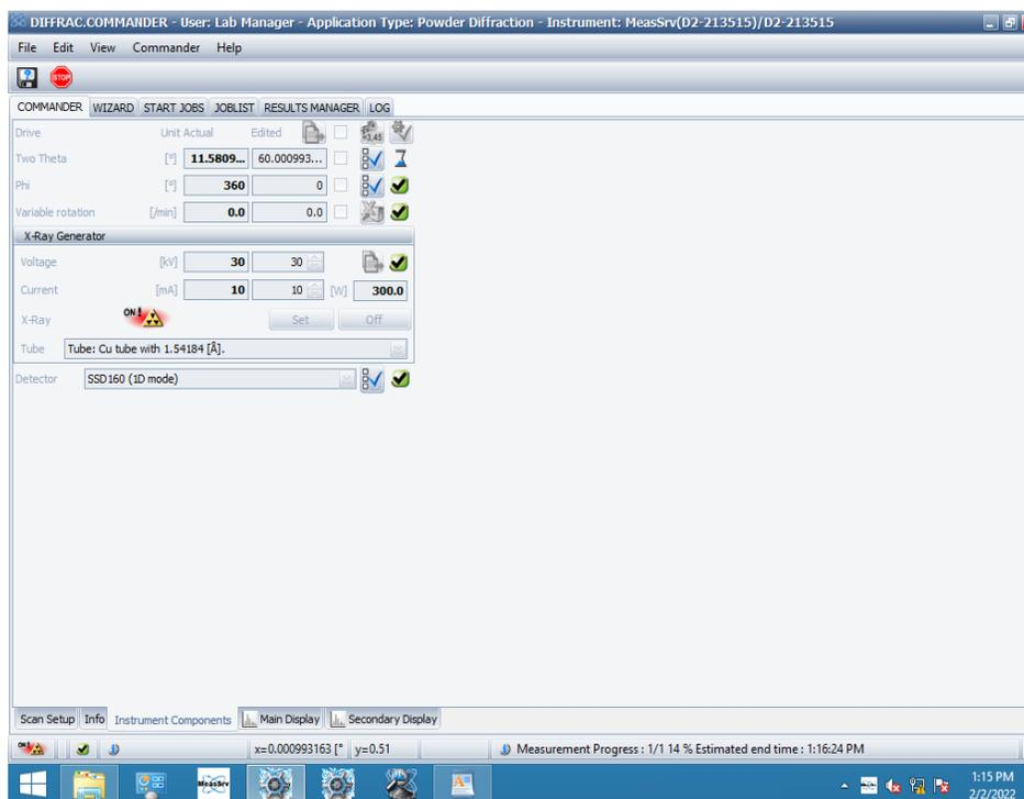
6.32 After a few seconds, you can begin to see the collection of data under the Main Display tab. A light on the interment will also indicate that it is busy and you will hear the instrument moving around as the data are collected.
