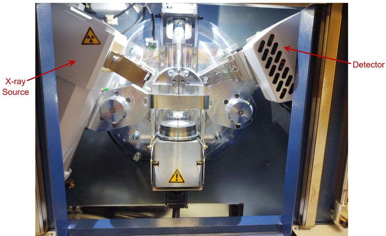
6.12 The sample is placed on top of the sample holder below.
