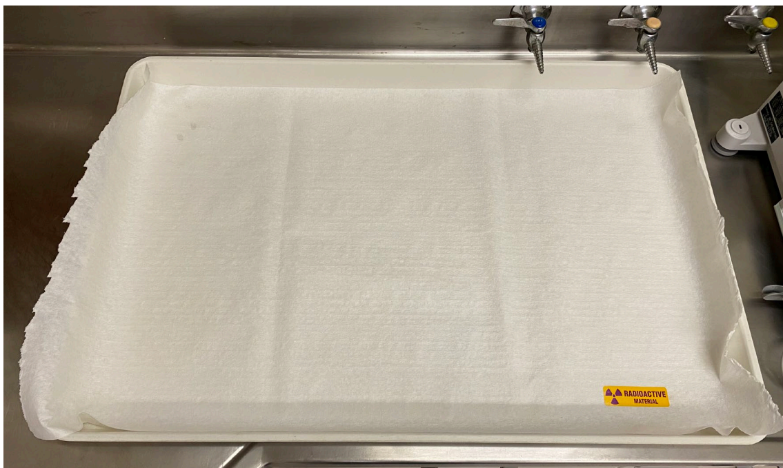
Figure 4-1. Lab tray system for use of radioactive materials.
