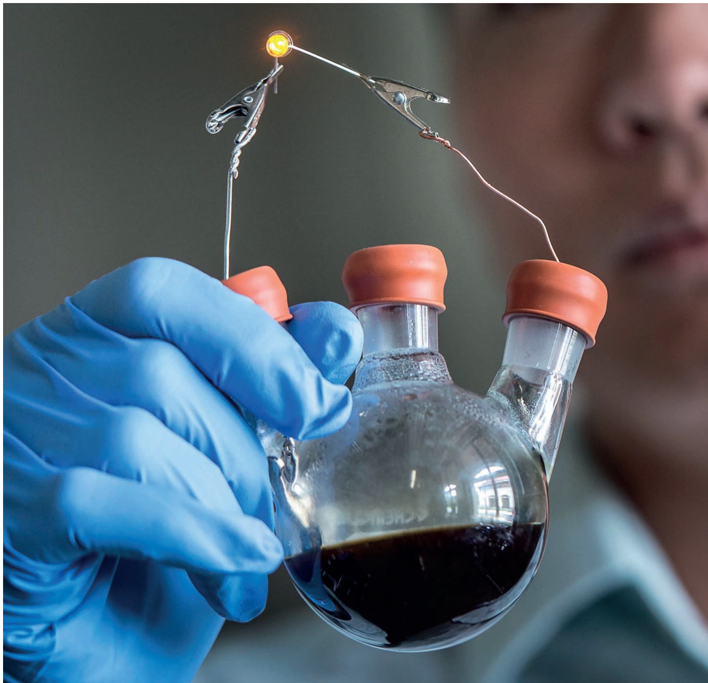
Industry funding supports more applied research, such as this lithium-polysulfide flow battery, which could serve as a model for low-cost, long-lasting energy storage.
