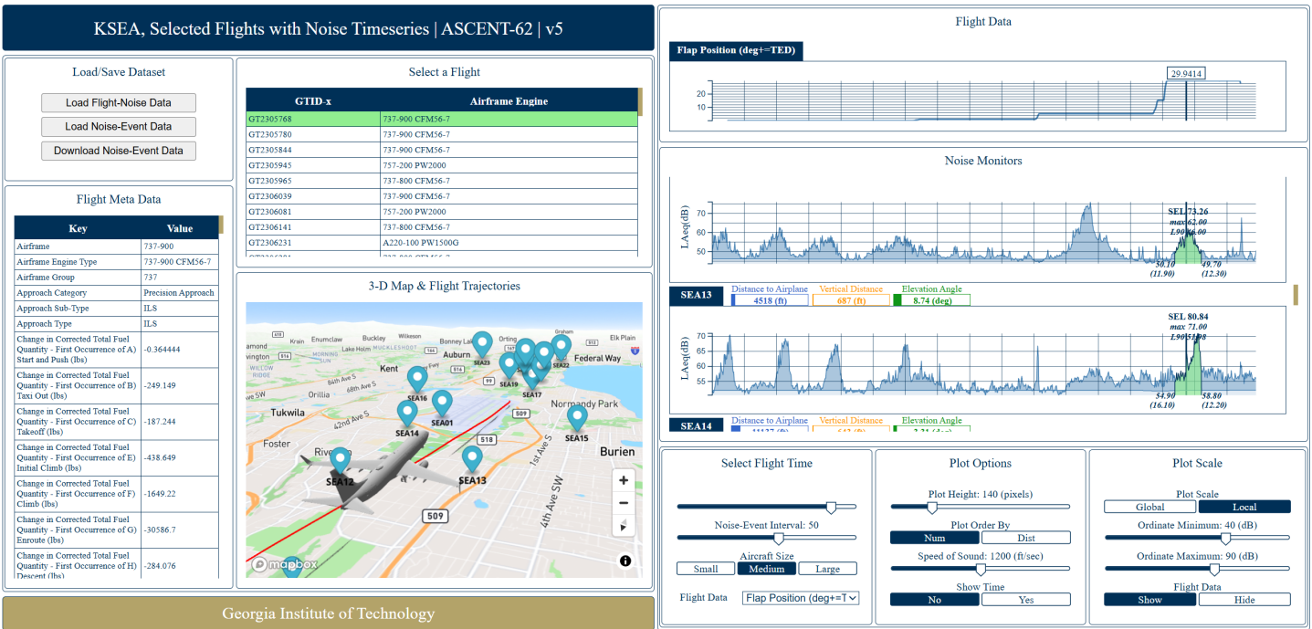
Figure 4. Interactive dashboard (v5) to capture sound exposure level (SEL) and maximum, A-weighted sound level ( L_{max} ) from Seattle-Tacoma International Airport (SEA) noise time history data.
