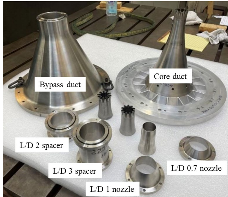
Figure 43. Model parts obtained from Gulfstream (Clemens & Gavin, 2024).
