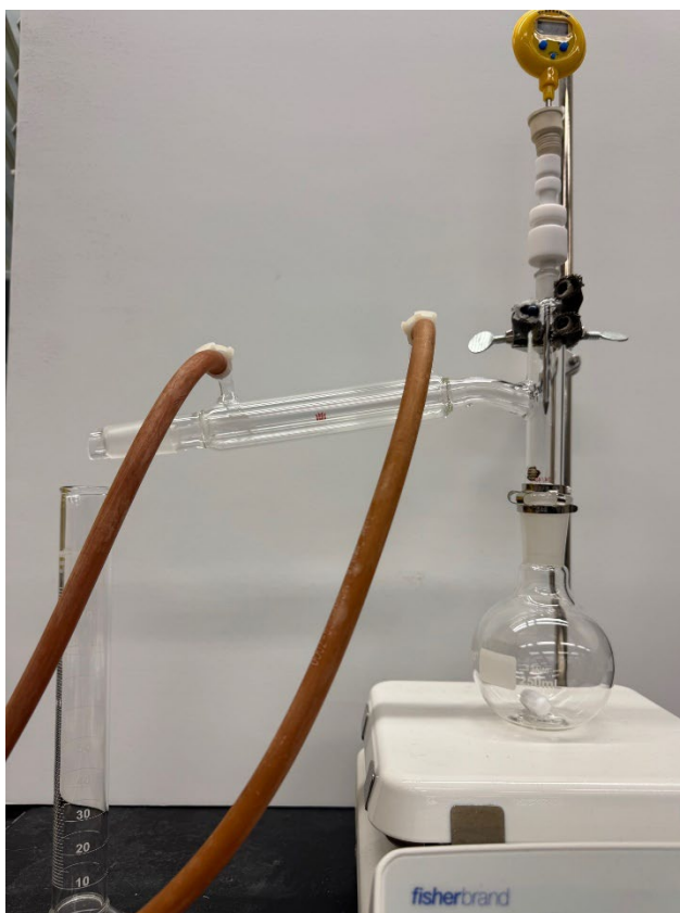
Figure 3. Apparatus used for distillations.
