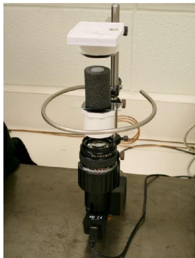
Figure 1. Schematic (left) and photograph (right) of an optical dilatometer.
