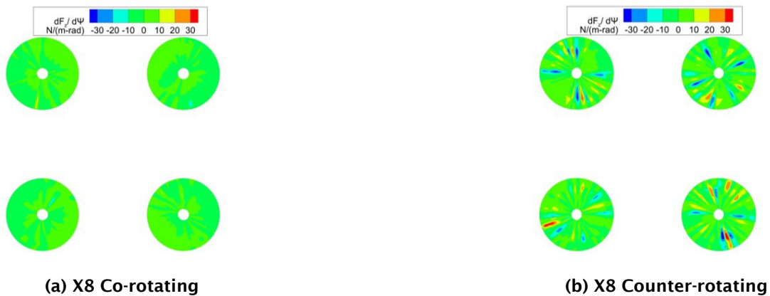
Figure 5. Variations in vertical force with respect to azimuth ( \frac{dF_z}{d\psi} ) during hover in rotor disk, (a) X8 co-rotating and (b) X8 counter-rotating.
