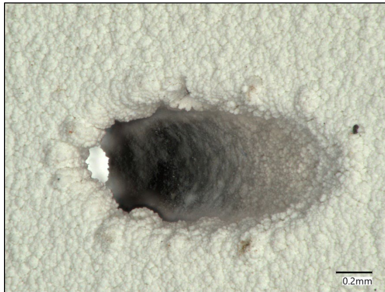
Figure 13. A hole on an effusion plate coated in yttria-stabilized zirconia thermal barrier coating.
