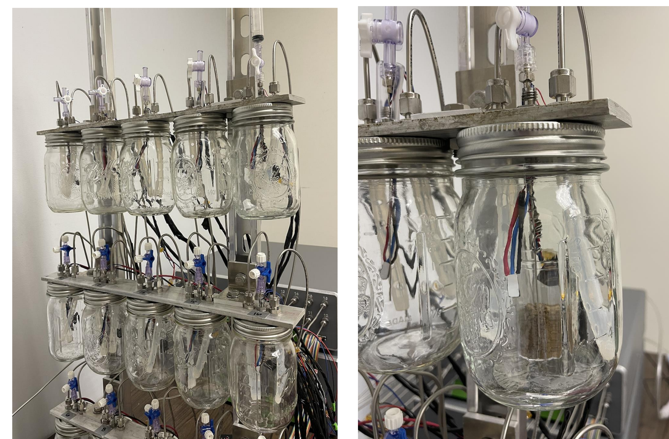
Fig 2. Laboratory incubation setup to trace carbon isotopes. Soil carbon and residue carbon are purposely selected to have different isotopic signature, C 3 and C 4 . Carbon dioxide from soil organic carbon and the decomposing residue from each jar is automatically measured every 5 hours with a Picarro G2121-i.
