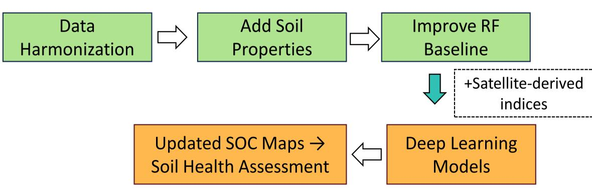
Harmonizing SOC datasets and adding soil properties improved model performance (validation  $R^2 = 0.74$  compared to 0.59 in previous work), emphasizing the importance of standardized data and enriched predictors.
