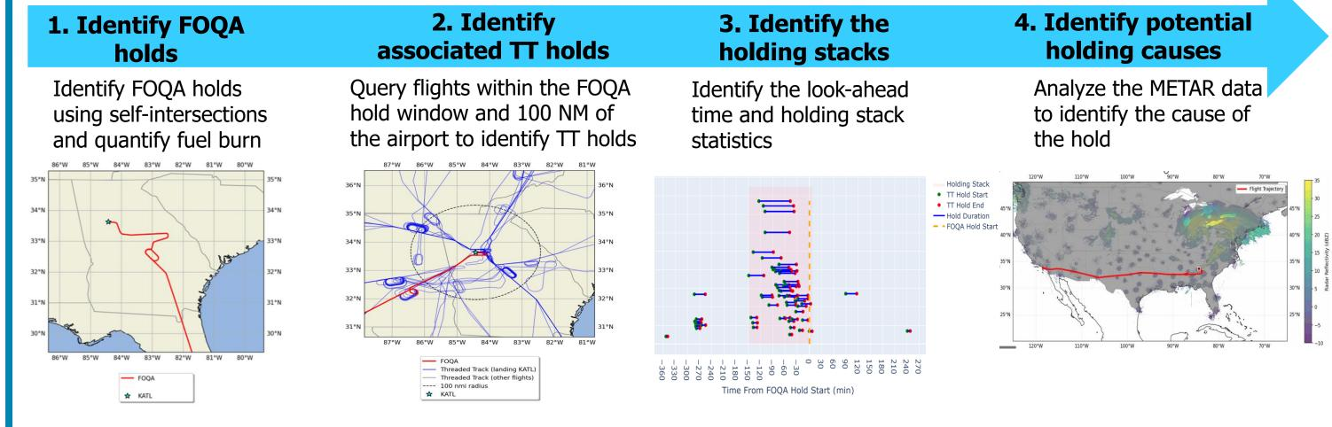
This analysis quantifies FOQA fuel burn during holding patterns, provides associated holding pattern statistics and determines the look-ahead time, which represents how early speed control can be applied in flight
