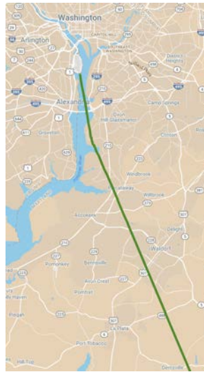
Figure 14. Ground track for departure procedure at DCA used in ANOPP and AEDT comparison.
