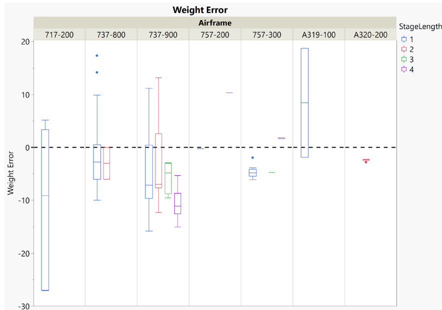
Figure 14. Aviation Environmental Design Tool (AEDT) weight assumption error ( \frac{\text{Weight}_{\text{AEDT}} - \text{Weight}_{\text{FOQA}}}{\text{Weight}_{\text{AEDT}}} * 100 ).
