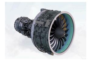
Largest broadband contributor in a fan stage is from rotor wake interaction with FEGV
