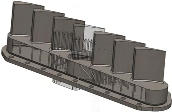
Figure 1. Example vane linear cascade with pressure tap design (the actual airfoils for this project are proprietary and therefore not shown).
