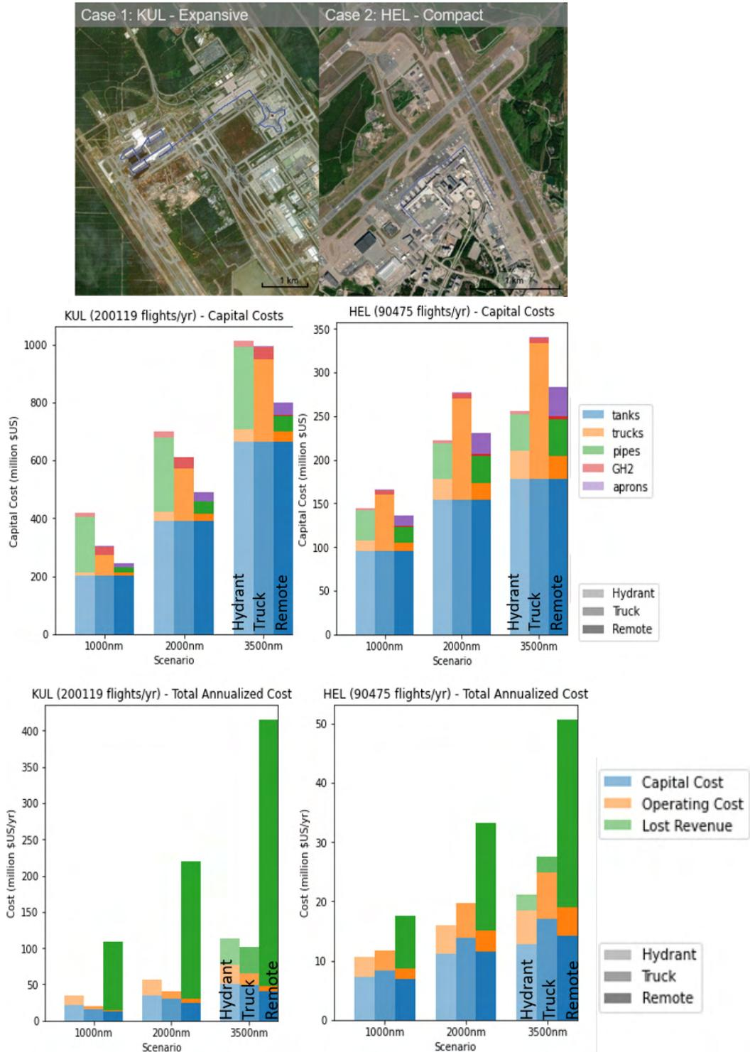
**Figure 8.** LH<sub>2</sub> airport distribution infrastructure case studies for Kuala Lumpur Airport (left) and Helsinki Airport (right), showing terminal layout (top), system CapEx (middle), and yearly annualized costs (bottom).
