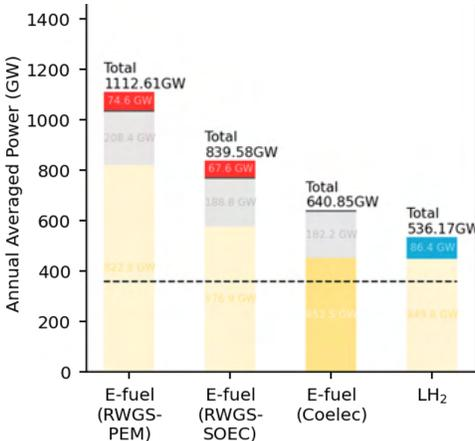
Figure 3. Energy system implications of replacing jet fuel with either LH<sub>2</sub> or PtL in a global replacement scenario (according to 2019 traffic).
