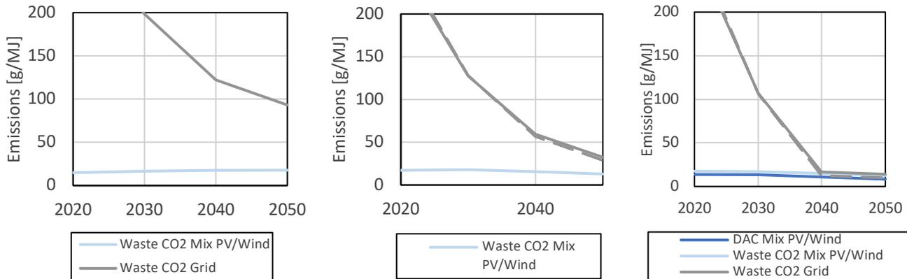
**Figure 6.** Emission trajectories of PtL production for three integrated scenarios reflecting different levels of ambition in the transition to a renewable energy base (left: least ambitious; middle: average scenario; right: most ambitious). Either waste CO<sub>2</sub> or atmospheric CO<sub>2</sub> is used for the production of PtL.
