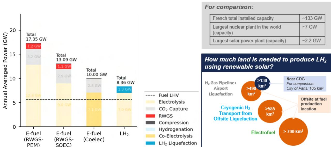
Figure 1. Energy system implications of supplying Paris Charles-de-Gaulle airport with LH<sub>2</sub> or PtL.
