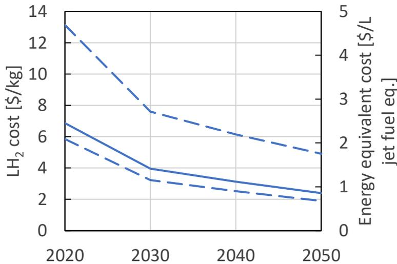
**Figure 5.** Minimum selling price of LH<sub>2</sub> fuel. Minimum, average, and maximum estimates are indicated.
