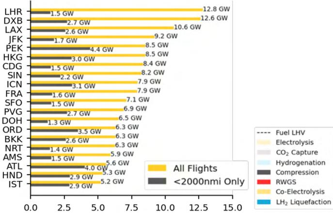
Figure 2. Energy system implications of replacing jet fuel with LH<sub>2</sub> at the 20 airports with the highest energy intensity (according to 2019 traffic).
