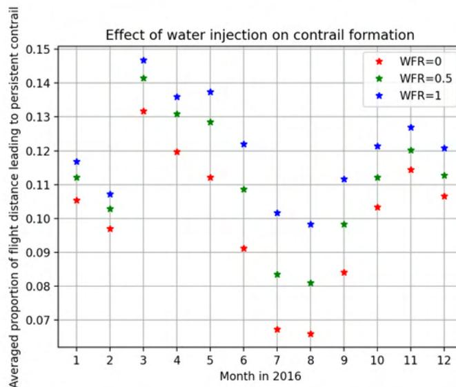
**Figure 6.** Effect of water injection on contrails.
