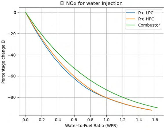
Figure 4. Combustor analysis: effect of water injection on  $\text{NO}_x$  emissions.
