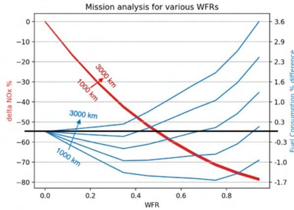
**Figure 5.** Overall mission analysis: effect of water injection on total fuel consumption and NO<sub>x</sub> emissions.
