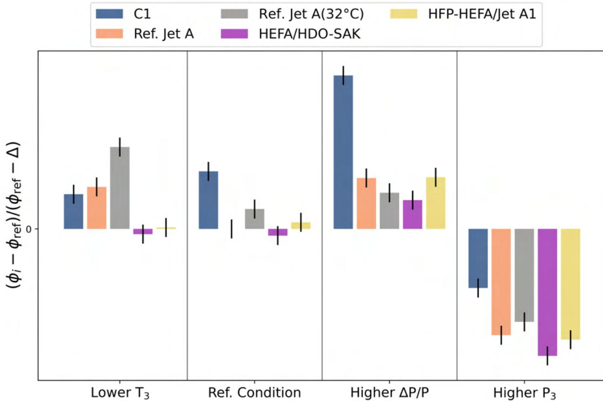
**Figure 4.** Relative lean blowout at four operating conditions in the GE9X full annular combustor rig. This figure was redrawn using data that was digitally extracted from the GE report to the FAA, which was part of the CLEEN II Consortium Program Update Public Plenary.
