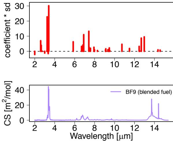
**Figure 4.** Wavelengths selected by the new strategy 1 model (based on 2- to 15-µm spectra) and their contributions to the variation in IBP (top); representative IR spectrum of BF9, a three-component hydrocarbon blend (bottom).
