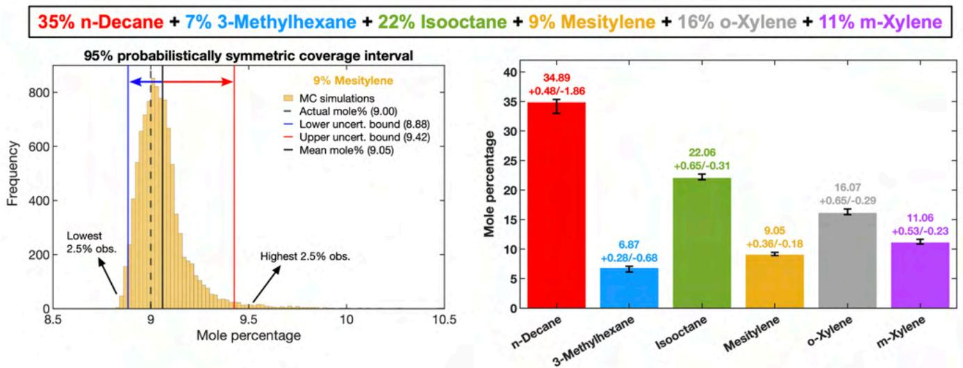
**Figure 5.** Strategy 4 uncertainty quantification for a simulated six-component mixture. Estimation of 95% confidence interval with Monte Carlo simulations for each component, shown here for mesitylene (left); estimated uncertainties in the mole percentages of the six components predicted with strategy 4 (right).
