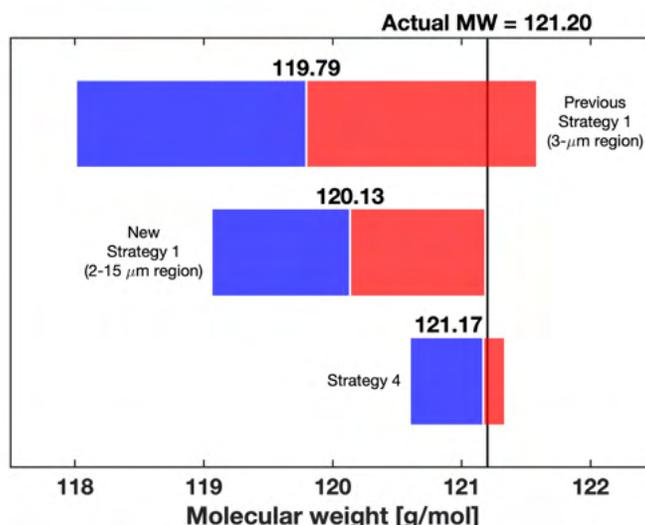
**Figure 6.** Comparison of uncertainty in the prediction of MW of the simulated six-component mixture by using the previous strategy 1 model (3- $\mu$ m region), the new strategy 1 model (2- to 15- $\mu$ m region), and strategy 4.
