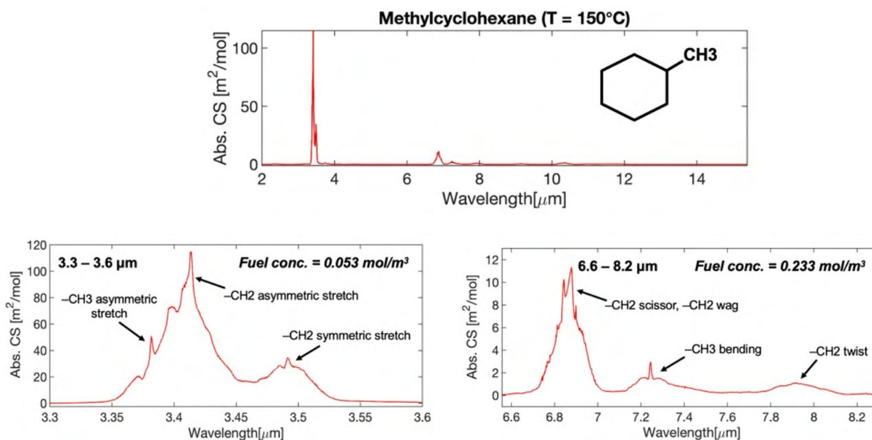
**Figure 2.** Measured 2- to 15- $\mu\text{m}$  spectrum of methylcyclohexane (top); strong -CH<sub>2</sub> and -CH<sub>3</sub> stretch features in the 3.3- to 3.6- $\mu\text{m}$  region, captured by using a using low fuel concentration (bottom left); relatively weaker -CH<sub>2</sub> and -CH<sub>3</sub> bending features in the 6.6- to 8.2- $\mu\text{m}$  region captured by using a high fuel concentration (bottom right).
