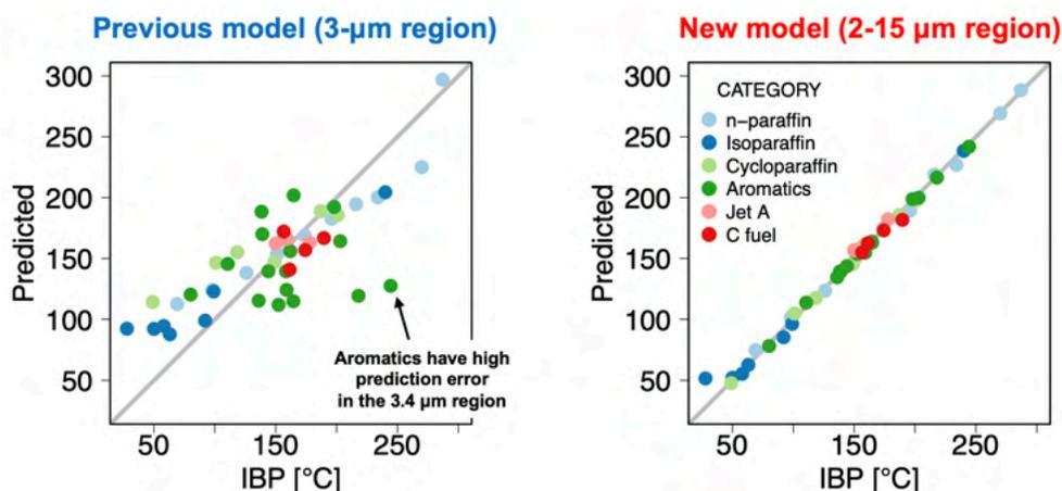
**Figure 3.** Actual versus predicted values of IBP by using strategy 1 models: previous model based on 3- $\mu\text{m}$  FTIR spectra (left); new model based on 2- to 15- $\mu\text{m}$  FTIR spectra (right).
