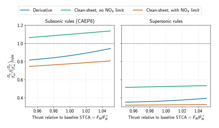
Derivative engine would meet the subsonic rules with a 6-16% margin
