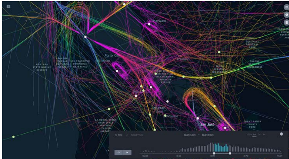
Figure 2. Current MONA web-access prototype for real-time aircraft location and 24-hr DNL contours.
