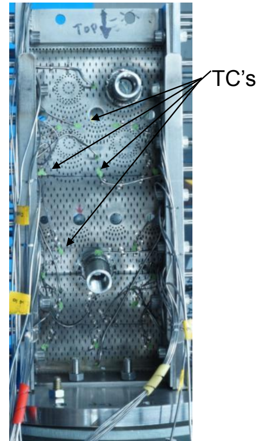
Top view of combustor
