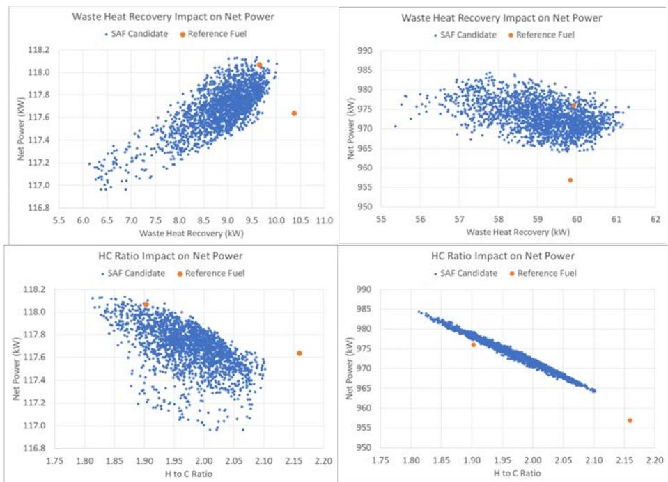
Figure 2. Main effects on net power from engine at low (left) and high (right) power.
