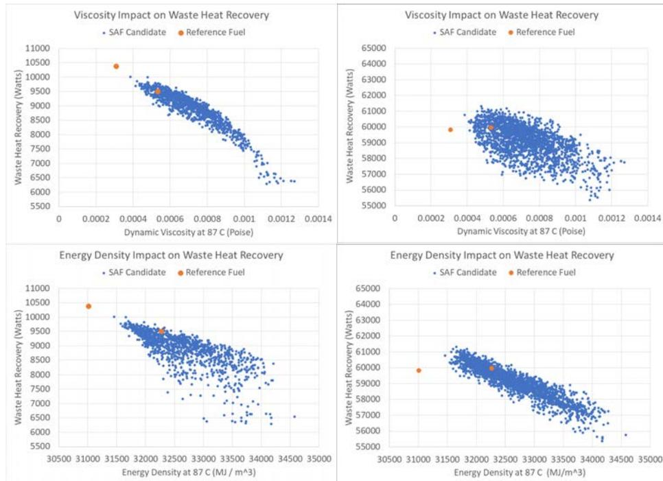
Figure 1. Main effects on waste heat recovery at low (left) and high (right) power.
