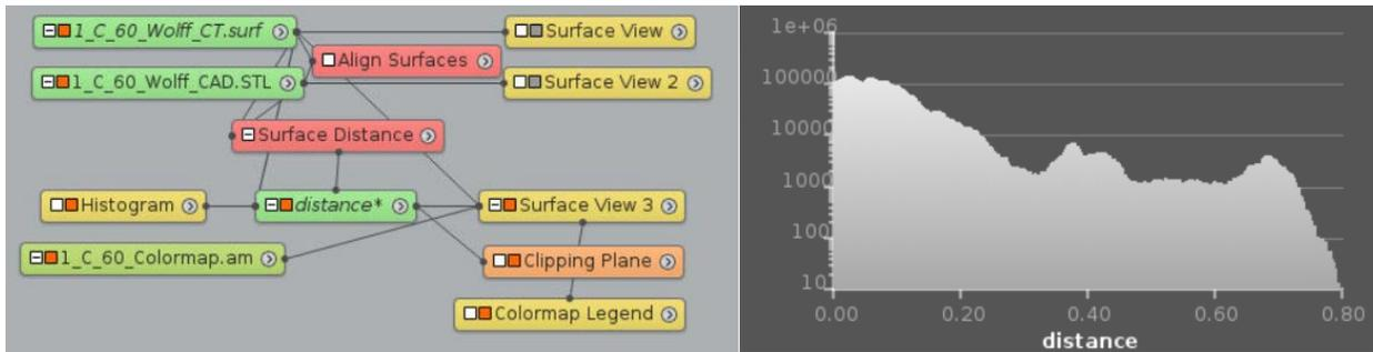
**Figure 4.** Steps performed in Avizo for a nominal-actual comparison, and the computed histogram of surface distance.
