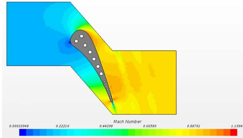
**Figure 7.** The predicted Mach number profile of the NASA C3X vane.
