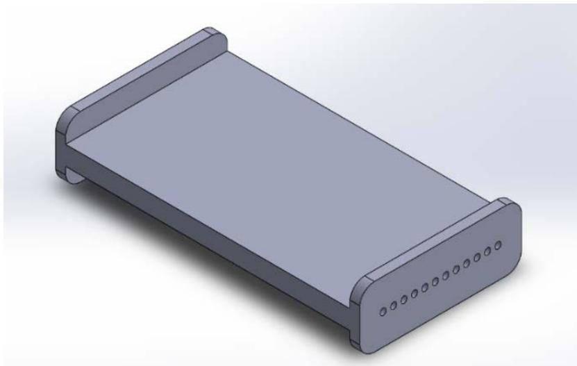
**Figure 2.** Solid body of the 1\_C\_60 public microchannel coupon in SolidWorks.
