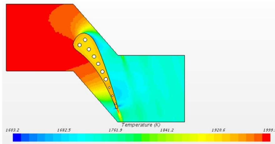
**Figure 8.** The predicted temperature profile of the NASA C3X vane.
