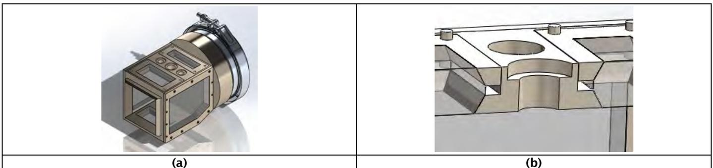
**Figure 3.** Combustor section showing: (a) liner with windows and frames, (b) “stepped” quench hole design.
