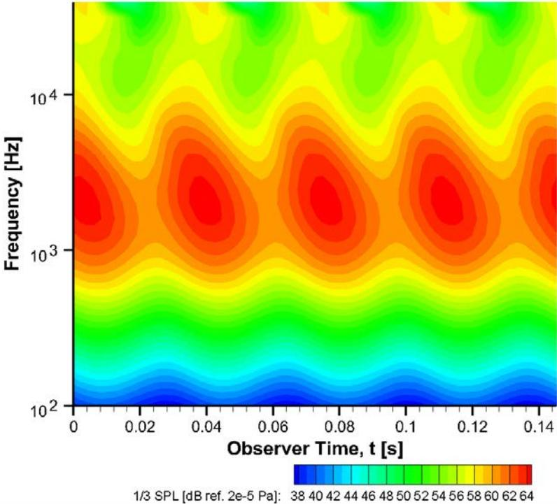
**Figure 9.** Spectrogram for observer located at  $-45^\circ$  elevation relative to hub plane,  $180^\circ$  azimuth, and distance  $11R$  from hub.
