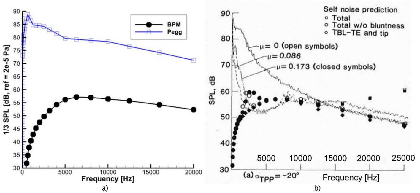
Figure 7. Broadband noise SPL spectrum for HART rotor case, advance ratio  $\mu = 0.173$ . a) PSU-WOPWOP prediction. b) Experimental data (lines) and ROTONET code predictions (symbols) (Ref. 3.2).
