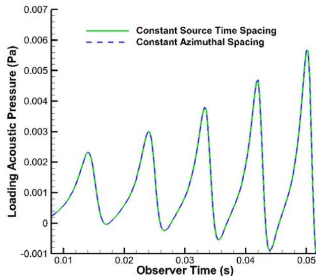
Figure 6. PSU-WOPWOP predictions for rotor with linearly increasing RPM.
