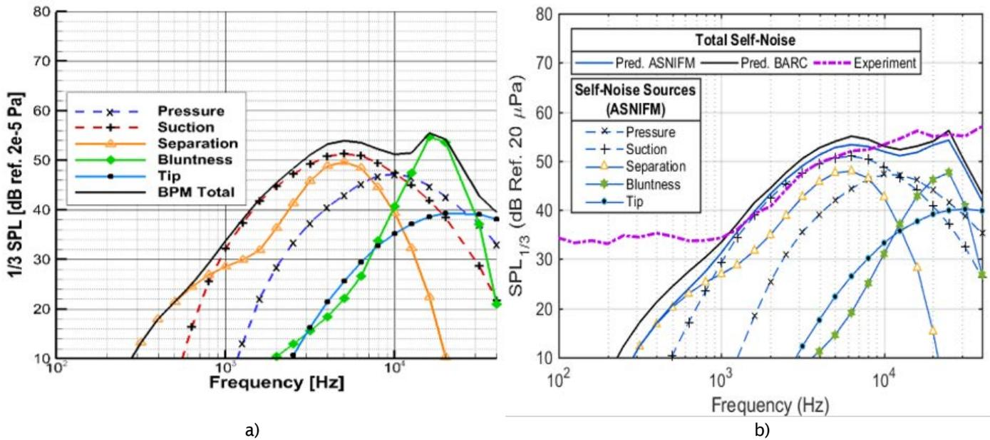
Figure 8. SPL spectrum from BPM model for ideally twisted rotor. a) PSU-WOPWOP prediction. b) BARC prediction (Ref. 3.3).
