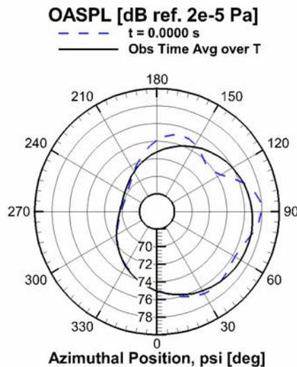
**Figure 11.** Broadband noise directivity in azimuthal plane, for observers located  $45^\circ$  below the tip-path-plane of the rotor, at a distance of  $11R$  from hub.
