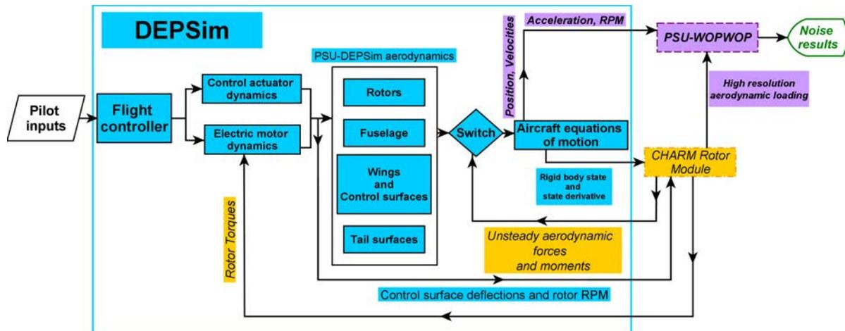
Figure 5. DEPSim system coupling schematic with CHARM rotor module and PSU-WOPWOP.
