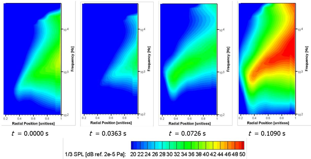
**Figure 10:** Observer time snapshots of spatial spectrogram of one rotor blade, for the same observer as Figure 9.
