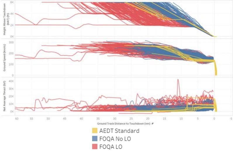
Figure 3. AEDT standard profiles next to FOQA data at KATL.
