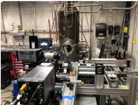
Figure 1. (a) Photographs of simultaneous PLIF and Mie imaging measurement system in VAPS test rig. (b) Schematic diagram of simultaneous PLIF and Mie system around the VAPS rig.
