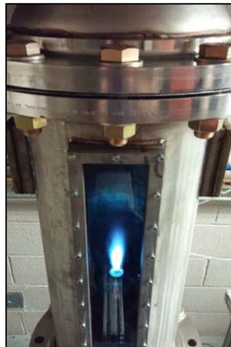
Figure 13. Picture of flame operating in pressure vessel at sub-atmospheric conditions.
