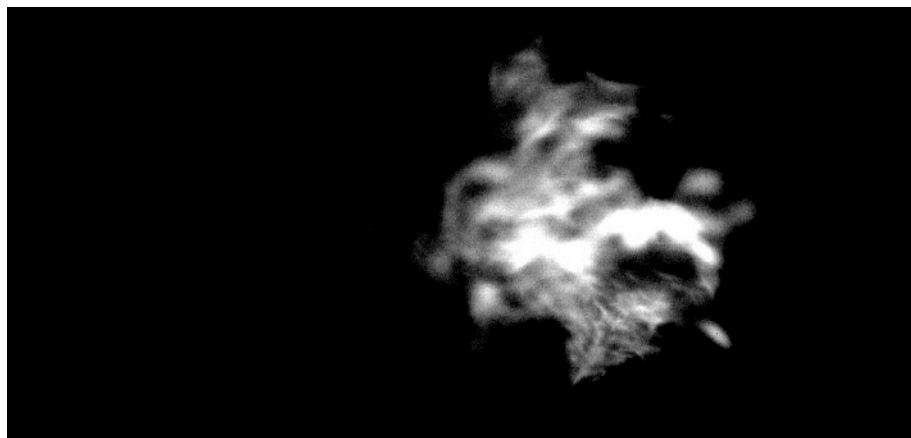
Figure 2. Sample flame chemiluminescence image from n-dodecane burning at 300 K air preheat temperature.
