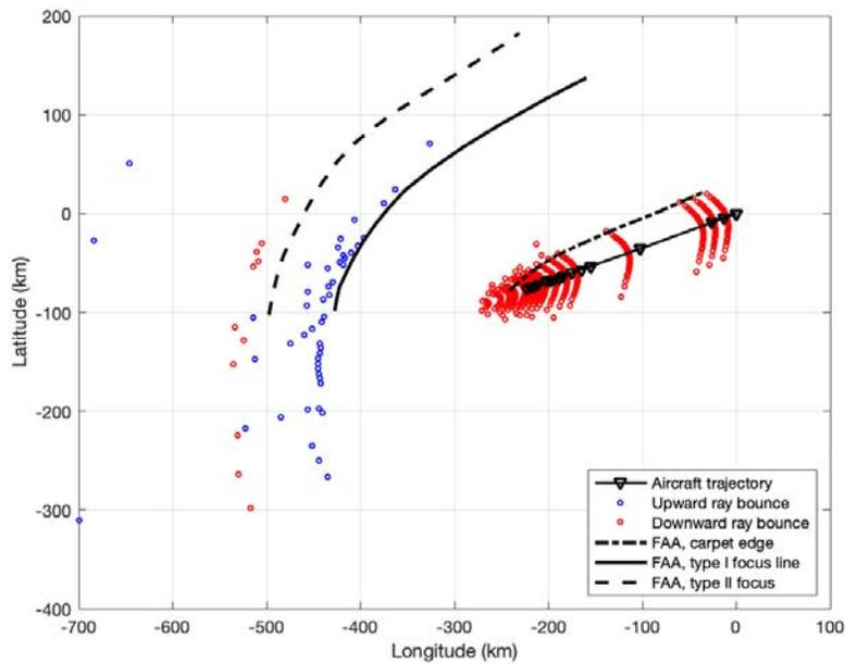
**Figure 9.** The secondary boom carpet with a spherical earth is shown with type I secondary sonic booms shown in blue and type II shown in red. The original focus lines from the 1980 Rickley and Pierce report area are shown in the figure as the solid and dashed black lines.
