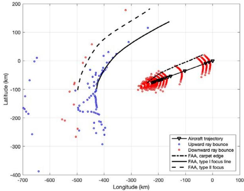
**Figure 8.** The secondary boom carpet for a flat earth approximation is shown with type I secondary sonic booms shown in blue and type II shown in red. The original focus lines from the 1980 Rickley and Pierce report area are shown in the figure as solid and dashed black lines.
