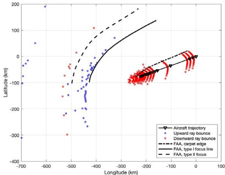
**Figure 10.** The secondary boom carpet with an ellipsoidal earth is shown with type I secondary sonic booms shown in blue and type II shown in red. The original focus lines from the 1980 Rickley and Pierce report area are shown in the figure as the solid and dashed black lines.
