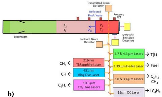
**Figure 1.** (a) Stanford 14-cm-diameter shock tube; and (b) schematic of shock tube/laser absorption setup. Simultaneous measurement of multiple species time-histories and temperature with microsecond time resolution are enabled using this arrangement (only a partial list of accessible species is indicated).
