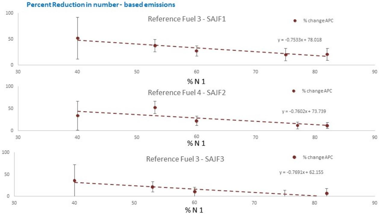
**Figure 3.** Example data of measured percentage reductions in particulate matter (PM) number-based emissions comparing blend emissions and reference fuel emissions. N1, rotational speed of the low-pressure compressor in a jet engine; APC, AVL particle counter (AVL, Graz, Austria).
