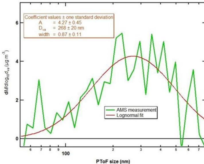
Particle size distribution (PSD) of organic PM (N1=82) is consistent with our previous study on lubrication oil emissions from aircraft engines (Yu et al., EST 2010)
