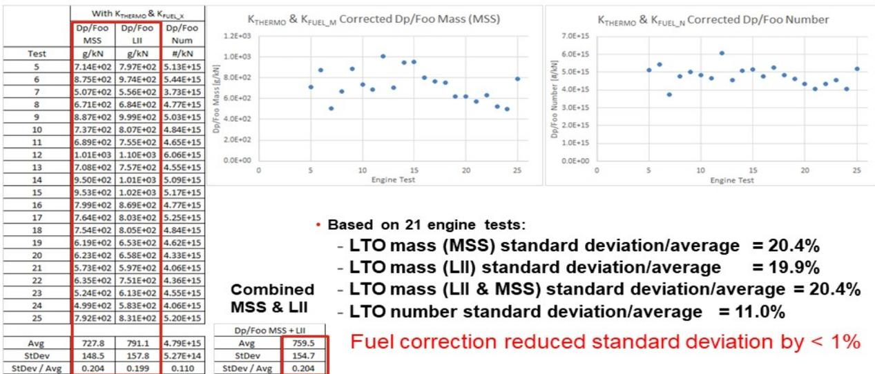
**Figure 1.** Summary of engine-to-engine variability data of 25 tests. nvPM, non-volatile particulate matter; LTO, landing and take-off cycle; LII, laser induced incandescence instrument; MSS, micro soot sensor; Dp/Foo, mass, in grams (Dp), of any pollutant emitted during the reference LTO cycle, divided by the rated output (Foo) of the engine.
