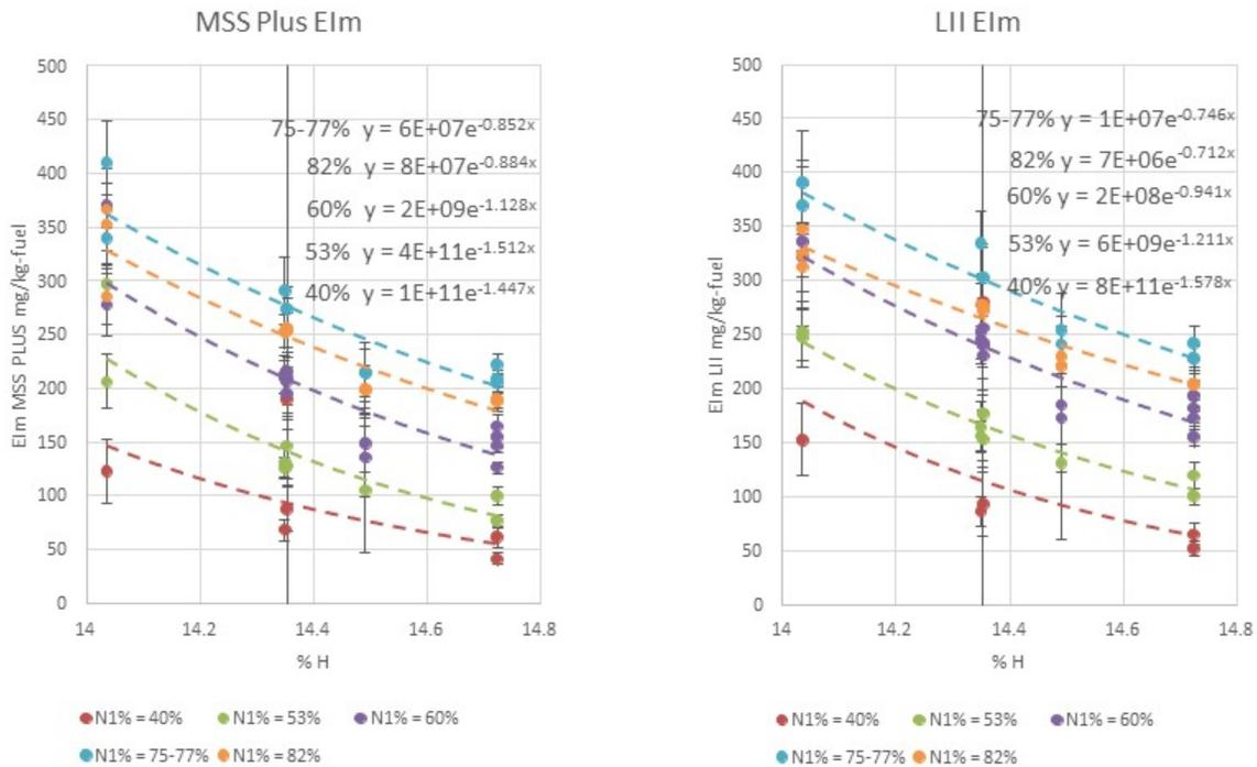
**Figure 4.** Example emission index values for the mass-based emission index ( $EI_m$ ) as a function of fuel hydrogen content (% H) using the micro soot sensor (MSS) and laser induced incandescence instrument (LII) mass measurement techniques.
