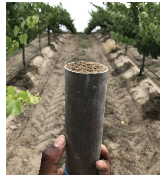
Figure 28. Soil scientists sampling soil bulk density in vineyards to quantify soil health. (Photo: Sarpong)
